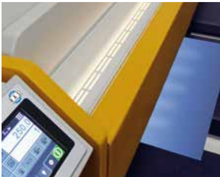
Convenient blank alignment to marks with the LED cutting line illumination.
